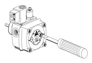
With the new Delta VU1 Universal pump it is now possible to substitute the pumps with shaft rotation clockwise and counter-clockwise, with delivery port on the right or on the left and one or two pipes system with only one unit, easily, and without special tools, the new pressure regulation gives a large pressure range without the necessity to change the spring.
