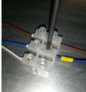
Join each one respectively to the new **BLUE** and **BROWN** wires of the 7-core cable using the 3 way terminal block. (NB. these wires are not polarity sensitive.).
