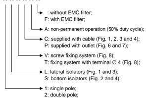
For instance, the designation TC2LVPAF indicates that the transformer belongs to the TC series, is provided with two lateral isolators, screw fixing system, power supply with outlet, EMC filter and is for non-permanent operation.
