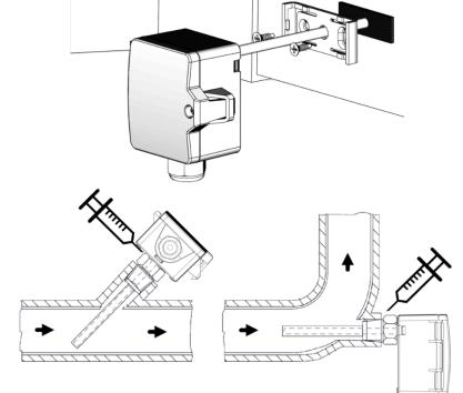
The sensor can be mounted on the ventilation duct by means of the mounting clip. For risk of condensate permeation in the sensor tube respectively in the immersion pocket the bushing must be installed in a position that occurred condensate can run off.
