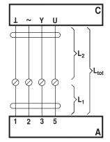
**Cross section** Max. cable length **Example for DC**  $L_2$  $L_{tot} = L_1 + L_2$ ⊥/~ AC DC  $0.75 \text{ mm}^2$ ≤40 m ≤20 m 1 m (L<sub>1</sub>) + 19 m (L<sub>2</sub>) 1.00 mm<sup>2</sup> ≤50 m ≤30 m 1 m (L<sub>1</sub>) + 29 m (L<sub>2</sub>) 1.50 mm<sup>2</sup> ≤80 m ≤45 m  $1 \text{ m } (L_1) + 44 \text{ m } (L_2)$  $2.50 \; mm^2$ ≤130 m ≤80 m  $1 \text{ m } (L_1) + 79 \text{ m } (L_2)$
