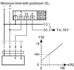
Override control with AC 24 V with Control remotely 0...100% with rotary switch
