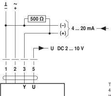
The 500  $\Omega$  resistor converts the 4 ... 20 mA current signal into a voltage signal DC 2 ... 10 V
