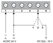
The actuator can be forced to override control when wired in acordance with the diagram.
