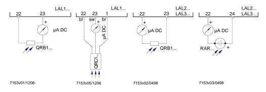
\* To comply with requirement of EN 230 clause 8.5 «Surge immunity test», for cable lengths above 10 m appropriate filter elements would have to be used. Experience has shown that filters are sometimes not necessary for normal operation even for cable lengths above 10 m.
